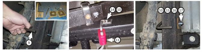
10. Route left front (4) and right tailpipes (6) over axle then connect them to muffler. Insert their wire hangers into isolators then tighten clamps just enough to allow for adjustment.
