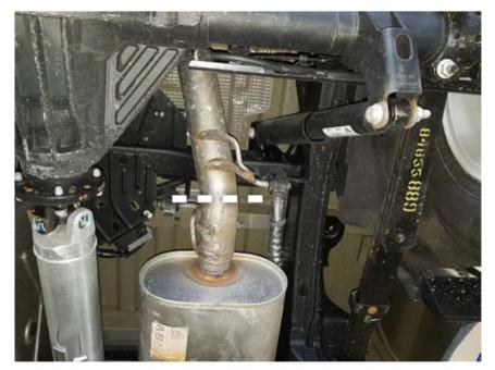
4. Support muffler and disassemble wire hangers from isolators. Remove and retain fasteners and gasket from flange, then remove muffler section from vehicle.
