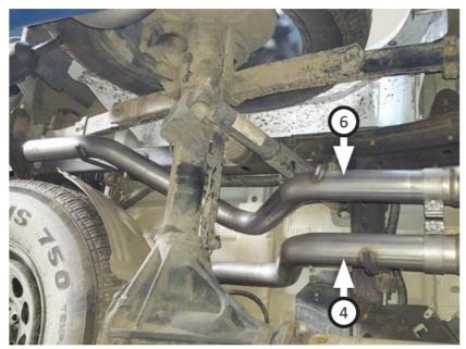
11. Place 2-1/2" clamp (12) onto left rear tailpipe (5) then connect it to left front tailpipe. Insert wire hanger into
