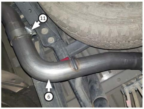
13. Place (x2 ea.) clamps (11) onto side exit pipes (7) then connect them to tailpipes and tighten clamps just enough to allow for later adjustment.
