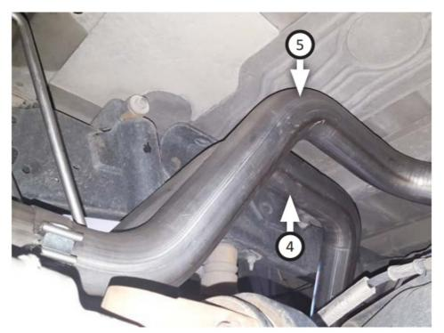
12. Place clamp (11) onto left rear tailpipe (6) and connect it to left front tailpipe. Insert wire hanger into isolator and tighten clamp just enough to allow for adjustment.
