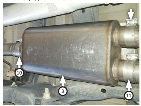
10. Remove bolts (x2) indicated below and use them to secure left rear hanger (9) onto vehicle frame. Then install rubber hanger (12) as shown.
