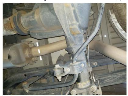
4. Support muffler and disassemble wire hangers from isolators. Loosen clamp, disconnect inlet pipe and remove exhaust system.
