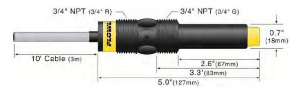
The sensor's operation may vary based on the dielectric properties of various application liquids. The LP15 series sensor is factory-calibrated to be used with liquids with a dielectric value between 20 and 80. Liquids with a dielectric constant less than 20 will not be detected by an LP15 series sensor.
