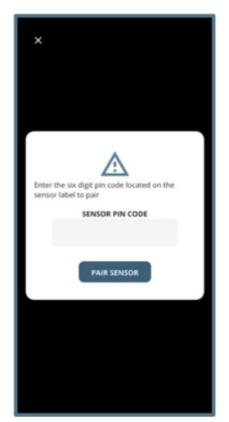
**Note:** The Sensor PIN Code will be the 6-digit manufacturer's date code located in the upper right corner of the label.
