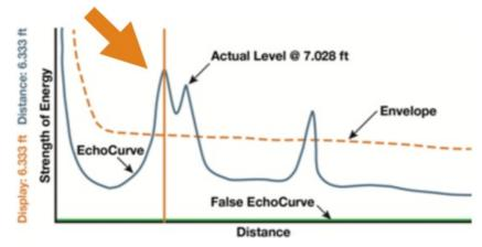
• If the most significant peak is ahead of/above the actual level of liquid or solids, this typically indicates
