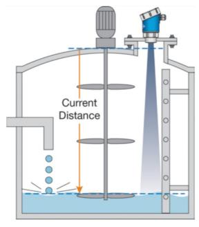
Obstructions in the tank (mixer blades, side wall weld joints, material build-up, submersible pumps, piping
