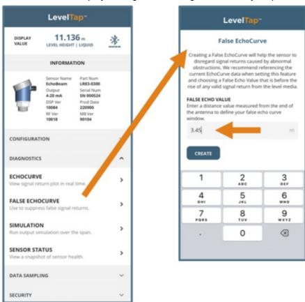
**Note:** To remove or undo the False EchoCurve, enter the value 0.001 and click on Create. This will erase the False EchoCurve
