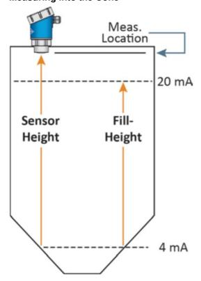
The sensor can read into the cone, but only to where most of the energy reflects to the sensor versus away from it.
