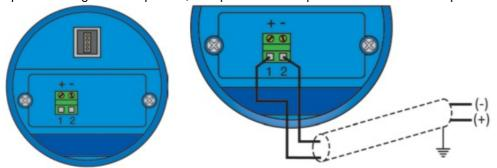
The Terminal (1) or Positive (+) and Terminal (2) or Negative (-) terminals are for connection to a 12-30 VDC power supply or to a 4-20 mA loop power source. The wire to the terminals can be extended up to 1,000 feet using 16-22 gauge wire.
