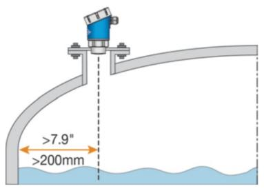
6. While adhering to the minimum free space requirements, based on the model, install the sensor with the following minimum distances away from the tank side walls:
