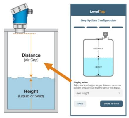
Press **WRITE TO UNIT** to save these settings in the transmitter. At this point, the EchoBeam® is configured to provide a 4-20mA signal proportional to the level in your tank.
