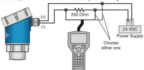
**Note**: The sensor should be wired with shielded 2-conductor cable (16 to 22 AWG) to protect from electromagnetic interference. If using a liquid tight connector, select a cable with an outer diameter that is designed to ensure an effective seal with the connector [typically between 0.20" to 0.35" (5 to 9 mm)].
