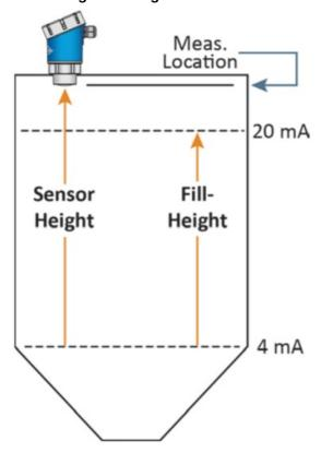
The sensor location is not critical because the lowest level reading is within the straight side wall of the tank.
