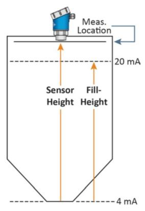
The sensor location is critical. The sensor must be installed over the lowest part of the tank to measure into the cone and to the bottom.
