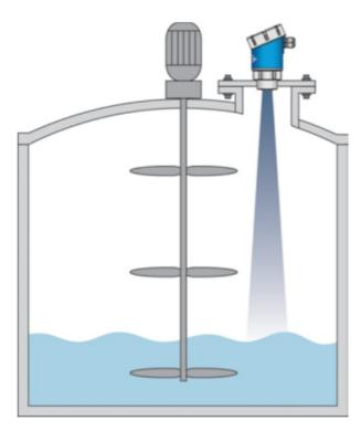
**Note:** EchoBeam® transmits a conical shaped RF measurement signal that spreads over a distance based on its beam angle. The below charts indicate the beam diameter or minimum free space required for each model at various measurement heights. If the sensor cannot be located away from obstacles that partially intrude into the beam diameter, perform a False EchoCurve configuration as described in Step 6.
