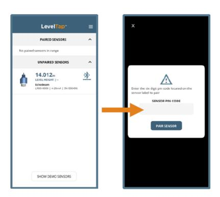
Note: The Sensor PIN Code is the manufacturer's date code located on the label of EchoBeam® (see below).
