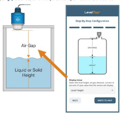
Press WRITE TO UNIT to save these settings in the transmitter. At this point, the EchoBeam® is configured to provide a 4-20mA signal proportional to the level in your tank.
