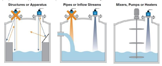
**Note:** EchoBeam® transmits a conical shaped RF measurement signal that spreads over a distance based on its beam angle. The below charts indicate the beam diameter or minimum free space required for each model at various measurement heights. If the sensor cannot be located away from obstacles that partially intrude into the beam diameter, perform a False EchoCurve configuration as described in Step 6.
