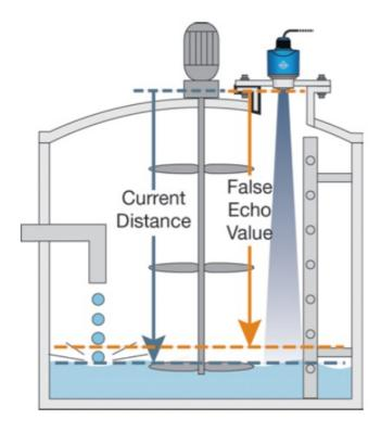
**Note:** A False EchoCurve should be performed when the tank is empty or as close to empty as possible. This is so all false reflections will be detected.
