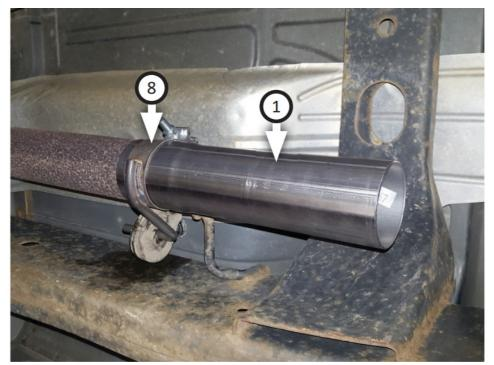
8. Place clamp (17) onto muffl er (2) then connect it to inlet pipe. Tighten clamp just enough to allow for adjustment then place (x2) clamps (16) onto muffl er outlets.
