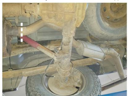
4. Support muffl er and disassemble wire hangers from isolators. Loosen ring clamp, disconnect inlet pipe then remove exhaust system.
