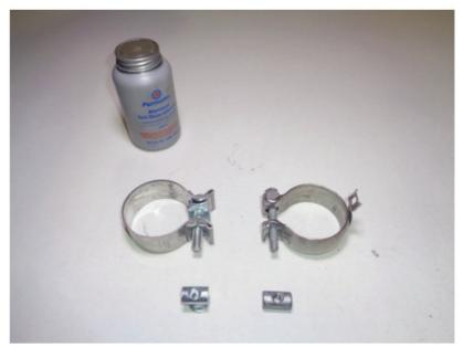
7. Place clamp hanger (8) to inlet pipe (1) then connect it to front pipe; lining inlet pipe notch up to front pipe tab.
