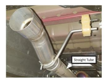
9. Place (x2) clamps (8) onto muffl er (3) then connect it to inlet pipe. Tighten clamp just enough to allow for adjustment.
