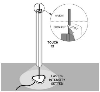
When the lamp is switched off, pressing once on the rod will light it up to the last programmed intensity. When the lamp is on, pressing once on the rod will switch it off.
