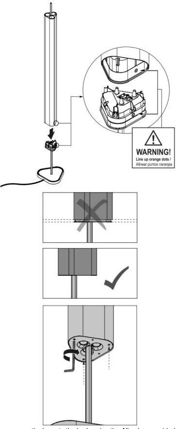
Before switching on the lamp, screw the base to the body using the Allen key provided with the product. Make sure that the screws are securely tightened and the diffuser is flush with the body.
