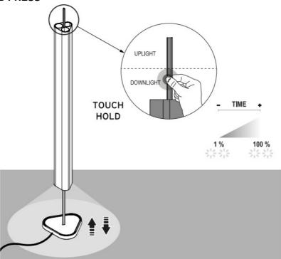
When the lamp is switched on or off, holding down the up or down rod will increase the intensity until it reaches 100% and the light will flash twice. By releasing and holding down on the up or down rod again, the intensity will be reduced until it reaches 1% and the light will flash twice.
