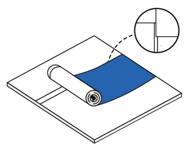
8. Remove the adhesive liner and adhere the foam to the film overlap.
