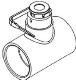
LEVERAGE To lift insert up and out
