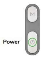
1. Press the power button briefly to turn on the Rangefinder. Look through the viewfinder to see the display. It will turn off automatically after 10 seconds.
