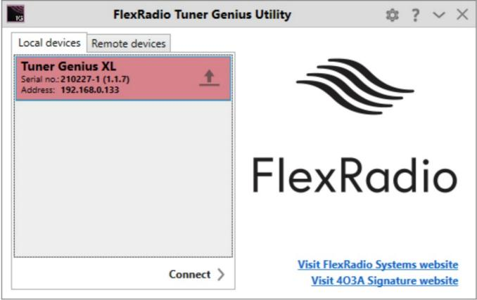
Caution: Never run previous versions of the Tuner Genius Utility with new Tuner Genius firmware. Before installing the latest release of the Tuner Genius Utility, you should remove any previous versions of the Tuner Genius Utility from all PCs on your network. Connecting an older version of the Tuner Genius Utility to a Tuner Genius ATU can result in unexpected and unreliable behavior.
