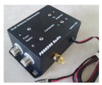
The Dual Antenna Disconnector by Paradan Radio is a good start but it will not survive a direct lightning strike. This device requires a switch 12V DC to turn on and off. If you use a Web relay to turn on and off your DC power supply then this can be wired directly to the power supply and ground your antennas when you turn off your station power supply.
