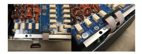
**Step 10:** Attach one end of the long coax cable to X6 of the LFP board below. Then route cable outside ribbon cables and attach the other end to X1 of the ETM board above. If the coax jumper is too short to reach the X1 connector the coax jumper can be routed on the inside of the ribbon cables. Be careful to insert coax connectors in straight to avoid damaging the center pin. You will hear a "click" when installed correctly.
