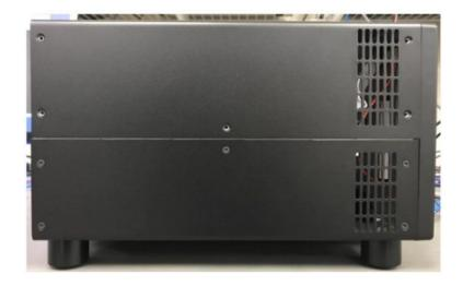
**Step 3:** Remove the top cover and handle gently so as not to scratch the cover. Set aside.
