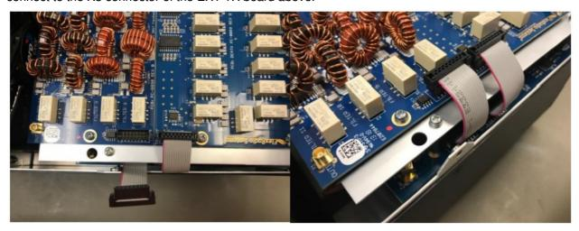
• Step 10: Attach one end of the long coax cable to X6 of the LFP board below. Then route cable outside ribbon cables and attach the other end to X1 of the EXT TX board above. (Be careful to insert coax connectors in straight to avoid damaging the center pin. You will hear a "click" when installed correctly.)
