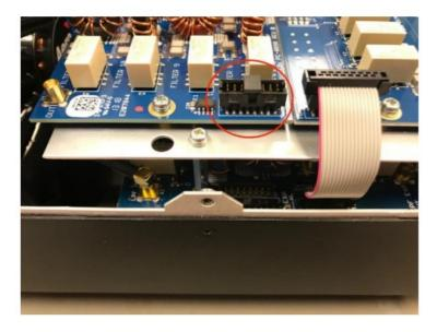
• Step 9: Connect the ribbon cable included in the kit to the X3 connector on the LPF board below first, then connect to the X3 connector of the EXT TX board above.
