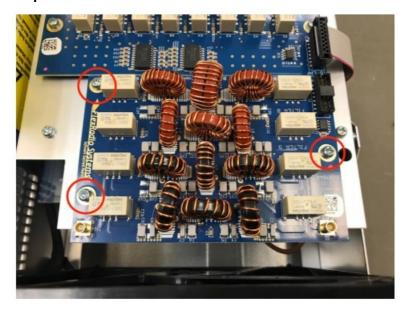
• Step 7: Connect the short coax cable included in the kit into the X1 connector of the LPF board below.
