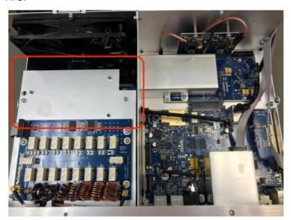
• Step 5: Remove EXT TX with the attached mounting platform from the bag. Remove the EXT TX board from the mounting platform by removing the three screws.
