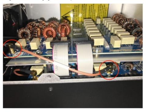
• Step 11: Replace the top cover being careful to not pinch the coax cable and screw it into place using 4 screws
