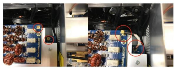
• Step 8: Remove plastic insert from X3 connector of EXT TX.
