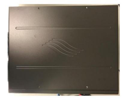
• Step 2: Carefully remove screws (5 each side) from both sides of the top cover using the T8 Torx.
