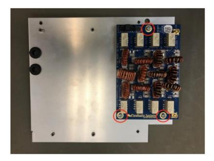
• Step 6: Install EXT TX in its location as shown with the three screws.
