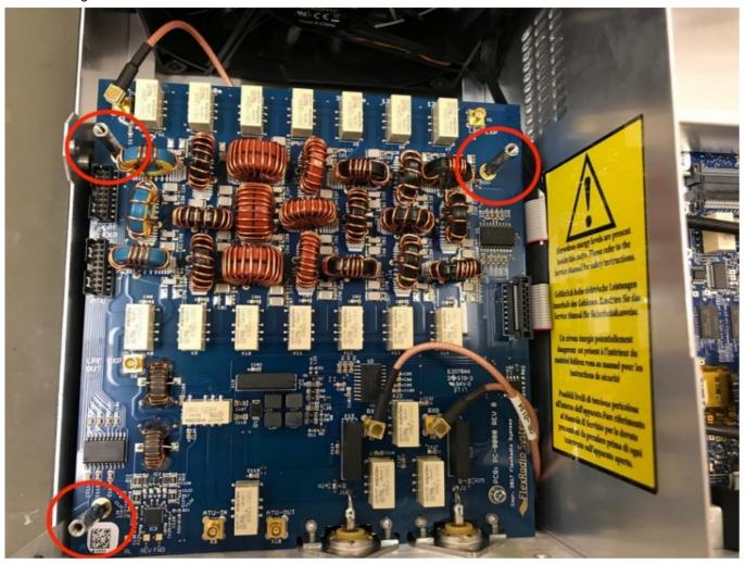
**Step 6**: Remove EXT TX with the attached mounting platform from the bag and place it on the standoffs with the holes aligned. Install the 3 screws that were removed to secure the EXT TX to the radio.
