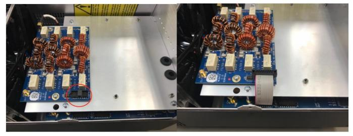
**Step 10:** Attach one end of the long coax cable to X6 of the LFP board below. Then route cable outside ribbon cable and attach the other end to X1 of the EXT TX board above. (Be careful to insert coax connectors in straight to avoid damaging the center pin. You will hear a "click" when installed correctly.)
