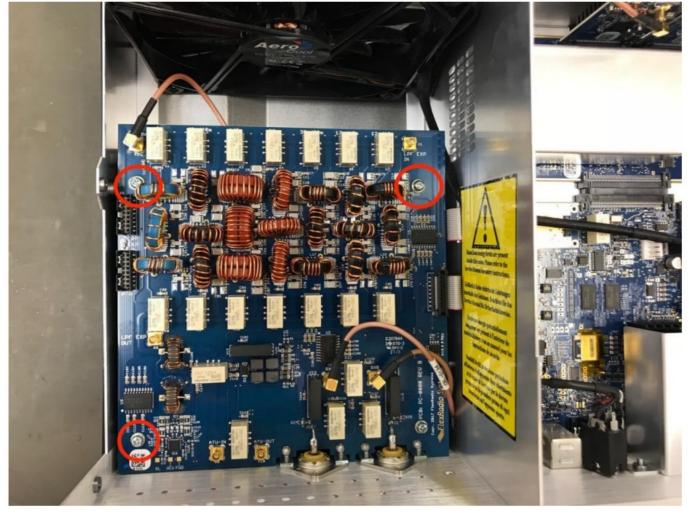
Step 5: Where the 3 screws were removed above, replace them with the 3 stand-offs included in the kit as shown
