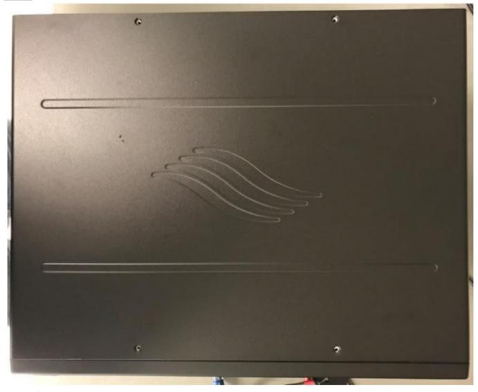
Step 2: Carefully remove screws (5 on each side) from both sides of the top cover using the T8 Torx.
