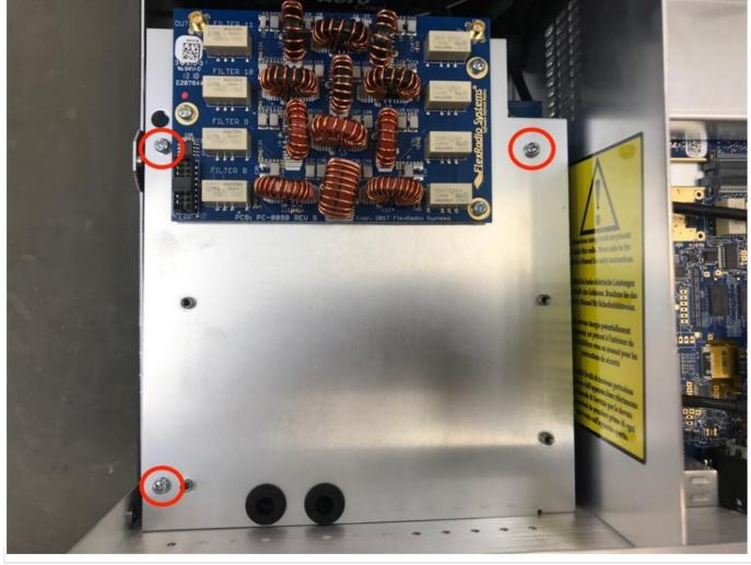
Step 7: Install a 4th screw included in the kit through the backside of the radio as shown below. It secures the mounting platform corner without a standoff.
