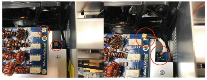
Step 9: Remove plastic insert from X3 connector of EXT TX. Connect the ribbon cable included in the kit to the X3 connector on the LPF board below first, then connect to the X3 connector of EXT TX board above.
