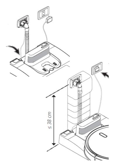
The connection cables must be positioned well and must not be squeezed under the charging station.
