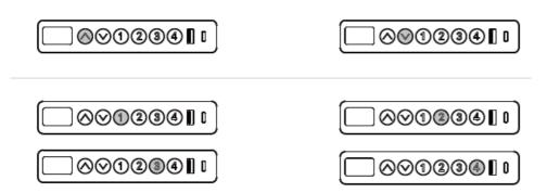
Press and hold the button "1", "2", "3" or "4" for 3s to save the current height
