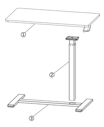
Step 1: Connect the lifting column to the tabletop
