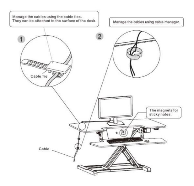
Do not tie the cables too tight. Allow the devices to move vertically to prevent property damage or personal injury.
