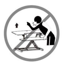
Lift the desktop to the top position before taking off the computer devices in order to prevent property damage or personal injury.
