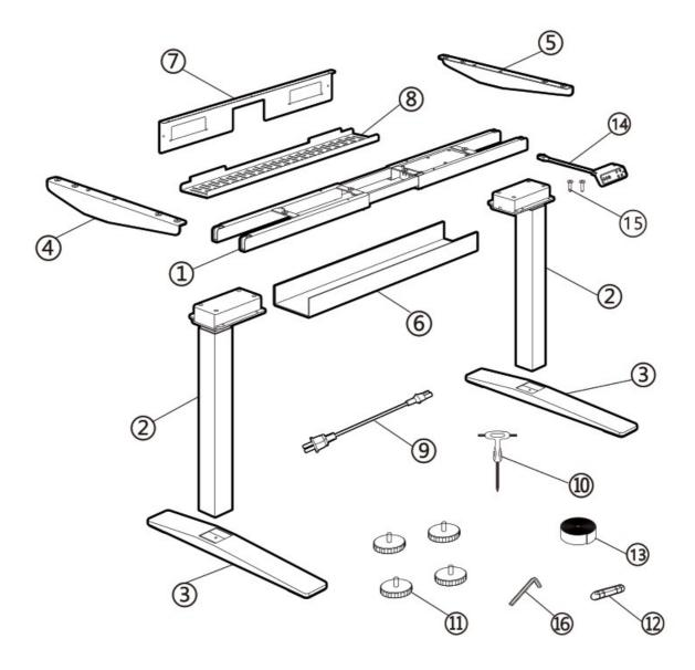
1. Attach the side brackets to the beam
