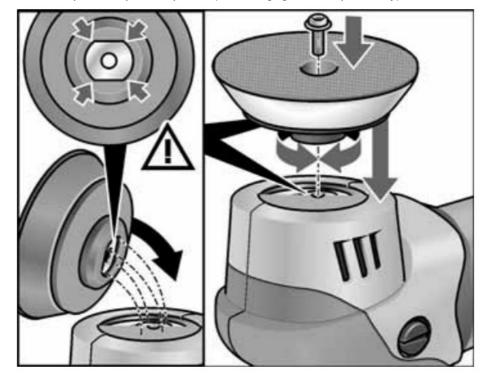
• Mount a new Velcro plate on the profile spindle. To do this, hand-tighten the hexagon socket head bolt in clockwise direction.
