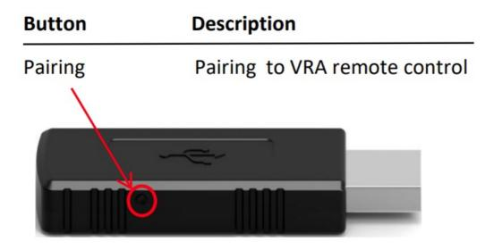
To pair the USB receiver with the VRA remote control
