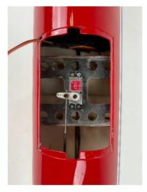
Make a slot as show in the picture below to allow the servo extension to pass through. Complete this section by closing the servo by with the cover supplied. Use a good quality clear tape. If you are super confident on your servo and installation you can apply clear silicone.
