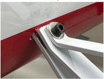
Once the front joiner and cross struts are installed on the fuselage, they will look like the pictures below:
