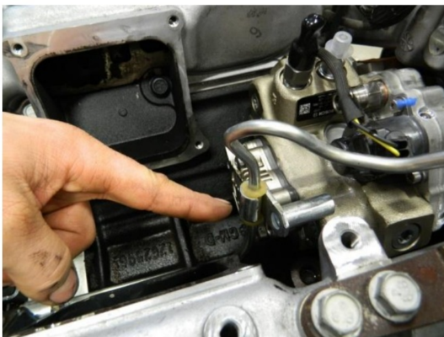
Carefully remove high pressure line bracket
