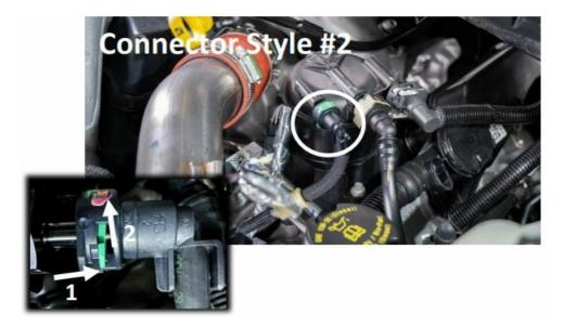
• STEP 3: Once the injector return connector is removed from the filter housing, use hose cutters or diagonal cutters to cut the fuel injector return line approximately one inch from the end of the fitting. Some installations may include the strain relief shown at right, which may be removed to expose additional hose.
