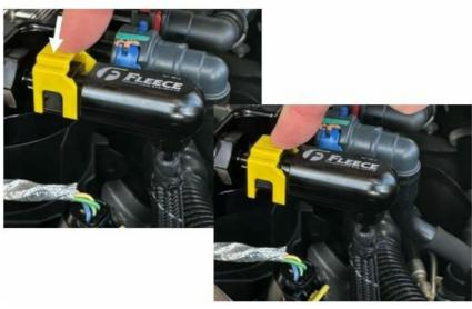
• STEP 10: Prime the fuel system by cycling the ignition to the on position without starting the vehicle. Verify no leaks are present. Start the vehicle and check for leaks.
