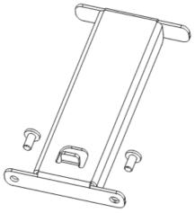
2. Install the spool holder at the position shown in the figure with the two screws. (Note: Please tighten them using a 2.0mm Allen wrench.)
