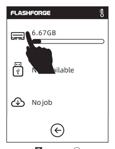
3. Locate the model file in the model list, Tap on its right to start printing; or tap the model file picture or file name to enter the model details page, and then tap to start printing.
