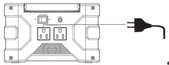
\*Note: When the AC port is not in use, turn off the AC power button to conserve
