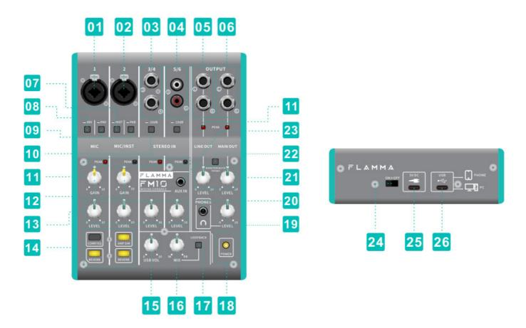
1. **Input 1-MIC/LINE:** XLR & 6.35mm TS input jack. Supports microphone (condenser microphone/moving coil microphone) or line input signal.
