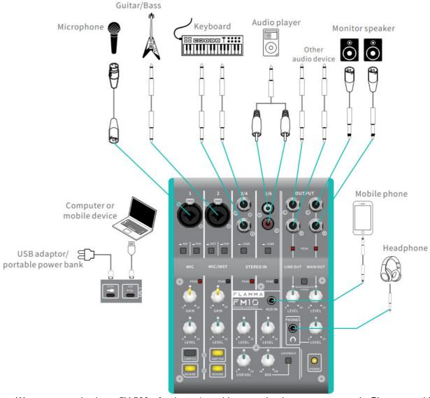
\*Notice: We recommend using a 5V 500mA adaptor/portable power bank as a power supply. Please use this port as a power supply if the connected device cannot power the FM10 via the USB port.
