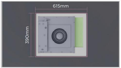
2. Create a 615x390mm cutout in the base of the cavity for the external blower. Ensure cutout is oriented correctly for selected ducting option.
