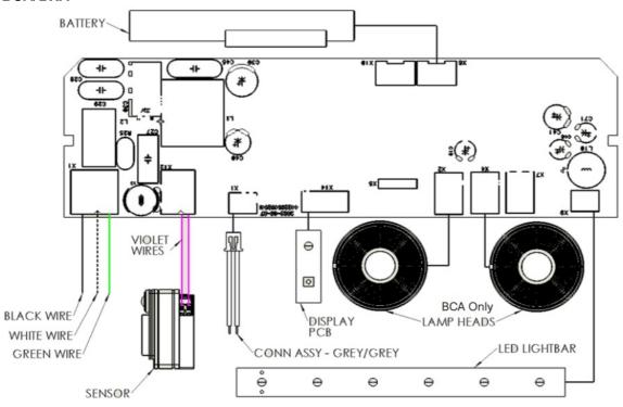
**NOTE** 1: For short-term testing of the emergency function, the battery must be charged for at least one hour. The emergency driver must be charged for at least 24 hours before conducting a long-term test.
