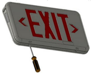
2. Remove center knockout in back plate and appropriate keyhole knockouts. Feed AC supply wires using screws provided center hole in backplate. Mount EXIT sign to junction box. **See Figure 2.**
