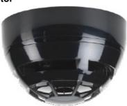
The WD200 wireless heat detector is able to signal the presence of a fire hazard based on the temperature detected in the environment. The detector is completely managed by the control panel (if combined with addressed control panels) and the single details relating to the status of the device are shown on the same. It can be set from the control panel as rate-of-rise (A1R) or fixed high temperature (BS).
