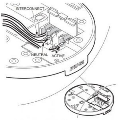
3. Clip terminal cover closed to avoid contact with live terminals.
