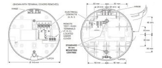
**NOTE:** Combined height of base and fitted smoke alarm: 52 mm.
