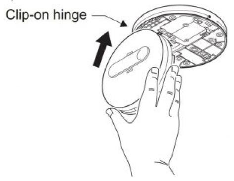
6. Use gentle pressure to latch the smoke alarm onto the base (take care to align the pins and terminals).
