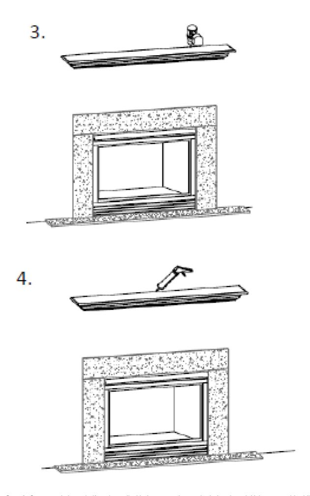
**Step 3**. Center and place shelf on the wall with the top resting on the ledger board. Using a portable drill, pre-drill three (3) or four (4) 1/16 inch holes down through the shelf top into the ledger board. The holes should be drilled 3/4 to 1 inch forward of the back edge of the shelf top equally spaced. Attach the shelf to the ledger board using
