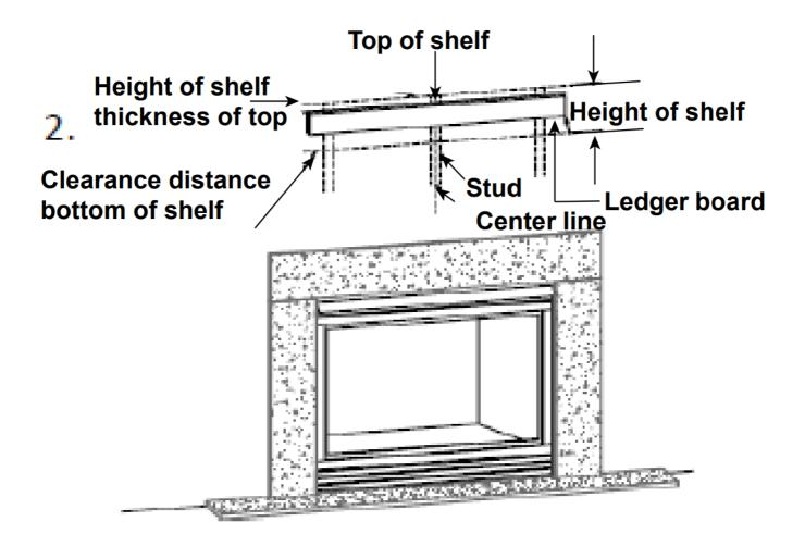
**Step 1**. Review mantel clearances found in the installation instructions included with the fireplace to determine the required distance from the top of the fireplace to the bottom of the shelf. Add the shelf height to the distance and mark on the wall with the pencil. Measure down the thickness of the shelf top and draw a level line approximately three (3) to four (4) feet long, depending on the shelf length.
