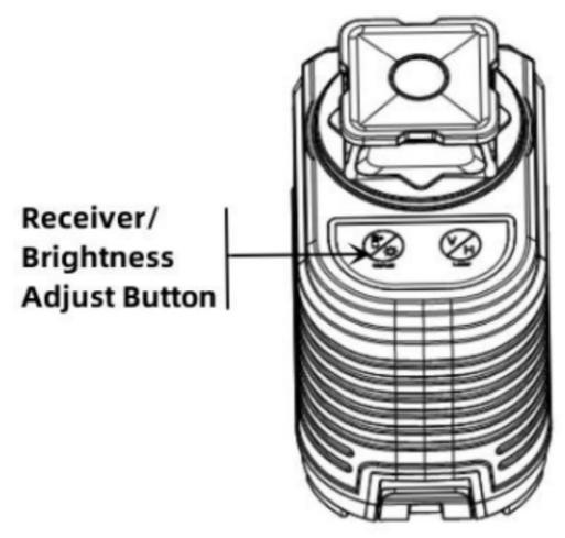
To switch to receiver (puse) mode, just single press the "Manual" button; then it goes to receiver mode.
