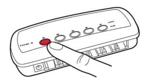
• With the Firecom Connect powered on, simultaneously push and hold the PWR and PTT buttons for 2 seconds, then release. The DECT LED light will blink green while pairing.
