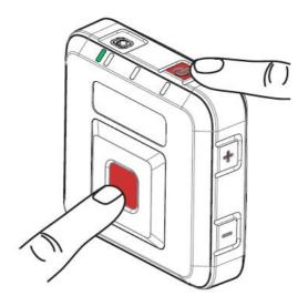
• The status LED will be solid green when connection is successful. If it is not, repeat the pairing process.
