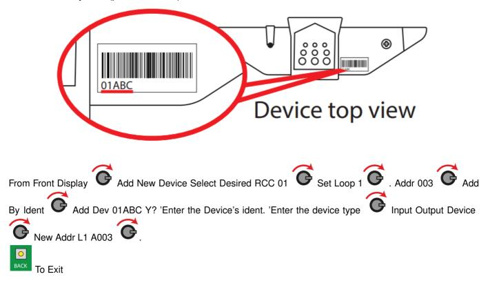
The device must now be assigned to the system. Refer to the 'Assign Devices' section on page 6 for details.
