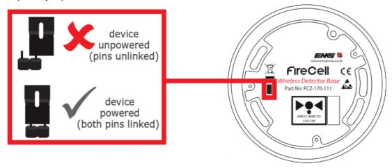
• Once powered, reassemble the device.
