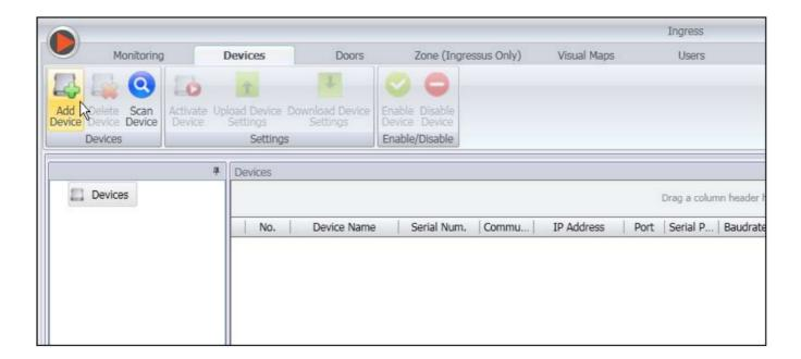
Once the door is added, click on Add Device at the Doors tab. Check/Tick the terminal(s) to be added to the specific door. Click OK. Double-click on the device. At the Network tab, click Edit. Change the desired IP address at the IP Address / URL column. When done, click Save to confirm the changes made.
