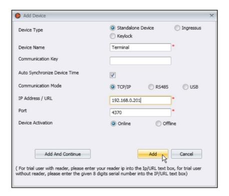
To add multiple devices at one go, click Scan Device and Scan. IP Address range can be set to search for devices. The bigger the range of IP addresses, the longer time needed to scan for devices. Devices found will be displayed on the screen. Select the preferred devices and click Add Selected Device to add them and a window containing the settings of the terminals will pop up. Click Add to proceed.
