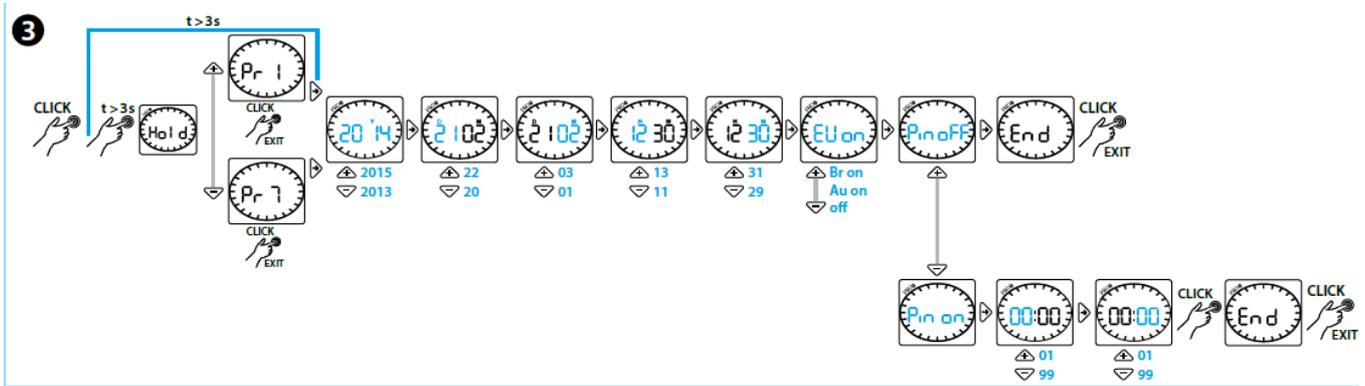
Push the joystick to activate the display. Push >3s to display Pr. Using the joystick set the following data:
