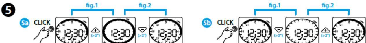
5a Push the joystick to activate the display. Push it towards the + symbol for 2 seconds to activate manual ON (fig.1). To deactivate, push the joystick towards the – symbol for 2 seconds (fig.2). 5b Push the joystick to activate the display. Push it towards the – symbol for 2 seconds to activate manual OFF (fig.1). To deactivate, push the joystick towards the + symbol for 2 seconds (fig.2).
