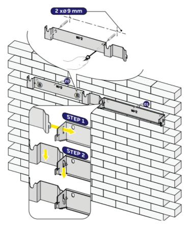
• Lift the REACT2-BATT(-5.0) up to the bracket and insert the heads of two anchor points (present on the back of the battery unit) into the slots on the bracket (20).
