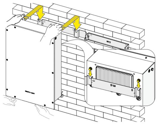
• Hang up the lower part of the REACT2-BATT(-5.0) to the wall using the two wall attachment point (26)(holes diameter 11 mm).
