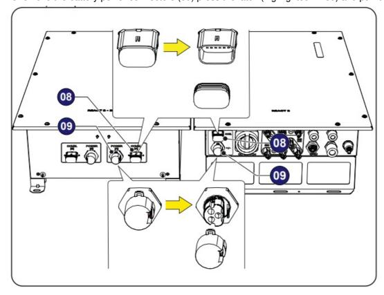
• Connect the two battery cables between inverter and battery unit (supplied inside the REACT2-UNO box).
