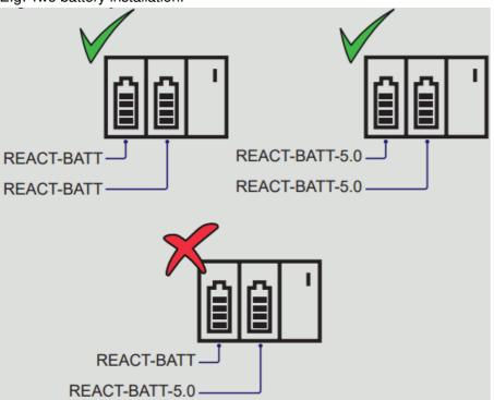
The principal components of the REACT2-BATT(-5.0) are shown in the figure and described in the following table:
