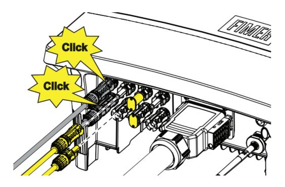
**ATTENTION** – Check that protective caps are installed on unused connectors. This is necessary for the inverter seal and to avoid any damage to the unused connectors which may be used at a later time.
