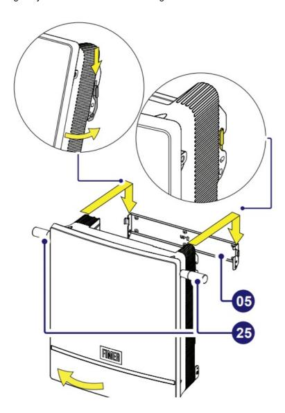
• Lift the inverter up to the bracket (05) (using the handles (25) or M8 eyebolts) and insert thetwo sides anchor
