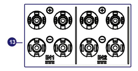
The input connectors are divided into 2 groups (one group for each input MPPT). For each MPPT 2 pairs of quick fit connectors are available.
