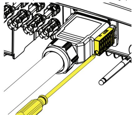
**ATTENTION** – The AC quick fit connector must not be subject to tensile forces (examples: do not connect weights to the AC cable, do not leave excess cable windings hanging, etc).
