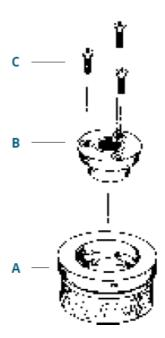
A. 52166 Body, WE-500N 52157 Body, WE-300N 52148 Body, WE-200N B. 52151 Insert Assembly, WE-500, 300N, and 200N C. 52152 Screw, WE-500, 300 and 200N
