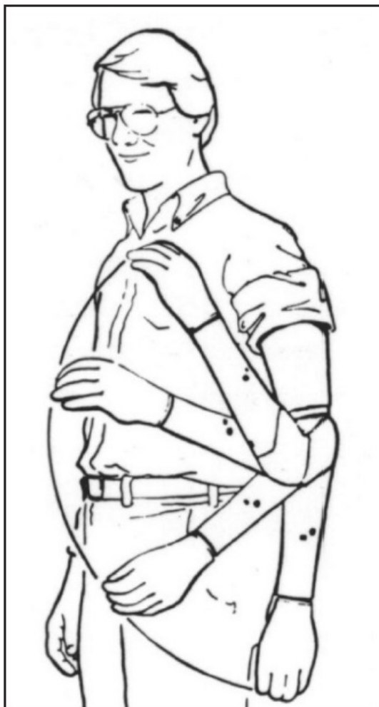
Figure 7 – Myoelectric Elbow Control; contract your “up” muscle to raise. Relax both muscles to lower with “Silent Freeswing”
