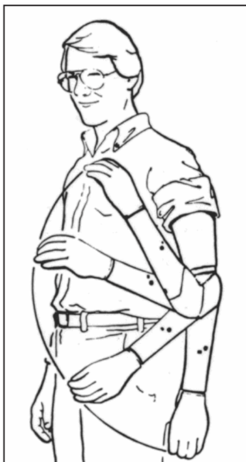
Figure 7 – Myoelectric Elbow Control; contract your “up” muscle to raise. Relax both muscles to lower with “Silent Freeswing”
