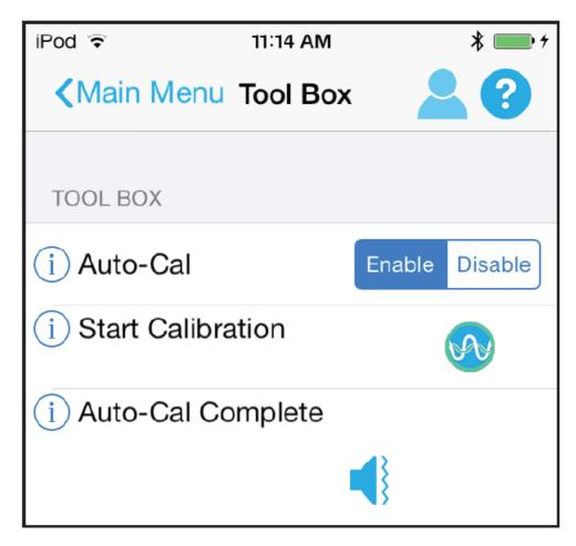
Auto-Cal is a feature on every ProPlus device. Use Auto-Cal only at the direction of your prosthetist. Triggering an Auto-Cal event will likely cause loss of the settings your prosthetist has programmed into your device.
