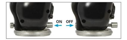
The power switch is located at the base of the ETD, on axis with the opening of the fingers. Pushing on the same side as the safety release turns the ETD ON. Pushing on the opposite side turns the ETD OFF.
