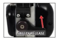
Pushing the safety release lever UP disengages the fingers, allowing the ETD to be easily opened.
