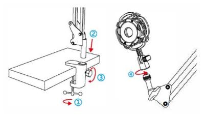
2. Install the Mic-Place the mic through the hold, then tighten the metal ring on the bottom of the shock mount.
