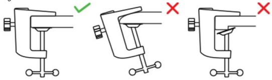
DON'T rotate the boom arm when the screw on the desk clamp is tightened. Loose the screw first, adjust the position of the arm, and the tighten it.
